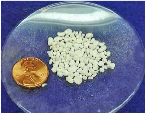
In most instances (though not all) our perlite is expanded in vertical furnaces. When the processed, unexpanded perlite is introduced into the furnace it falls down towards the heat source. As it falls it begins to expand becoming buoyant in the air stream running through the system. The furnace operator can control the density of the finished product by adjusting the temperature and air flow in the furnace.
